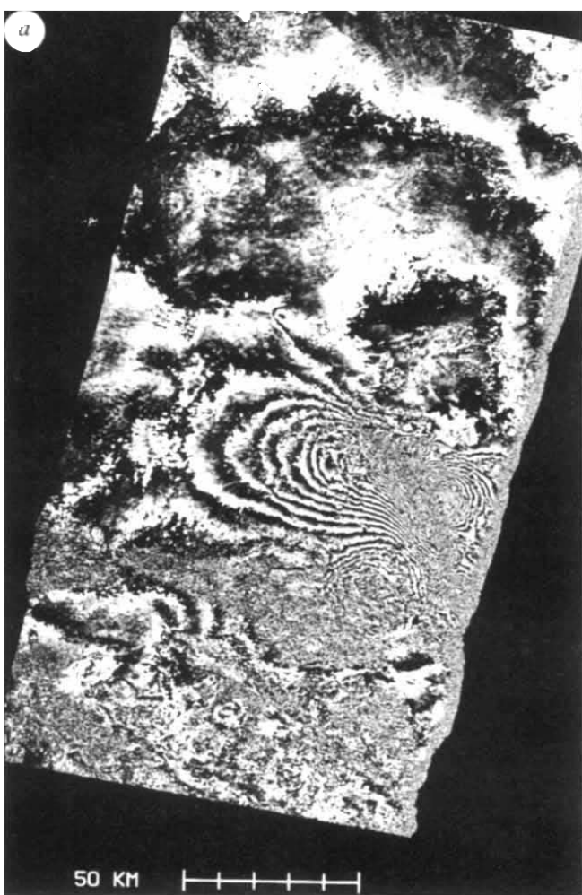
FIG. 2 a , Post-processing interferometric fringes obtained with the pair of ERS-1 SAR images taken before (24 April) and after (7 August) the earthquake. The image covers the 125 by 275 km area outlined by the large rectangle in Fig. 1. One cycle of gray shading represents a range difference of 28 mm between the two images. It is a measure of the component of the displacement vector which points toward the satellite. The number of fringes increases from zero at the northern edge of the image, where no co-seismic displacement is assumed, to at least 20 (representing 560 mm in range difference) in the cores of the lobes adjacent to the fault. The asymmetry between the two sides of the fault is due to the curvature of the fault and the geometry of the radar. Displacements with different azimuths on opposite sides of the fault produce different fringe patterns because the radar resolves only the range component of the displacement vector. b , Detail of the fringe map in a , covering an area 64 km by 33 km as outlined by the small rectangle in Fig. 1. The orbital separation, or baseline, between the images taken 24 April and 7 August measures approximately 60 m and 126 m, in the vertical and horizontal components respectively. These values imply that an error in the elevation model of 72 m would produce a shift of one full cycle. c , Fringes obtained using the same processing and area for b , but with SAR images acquired on 3 July and 7 August (after the 28 June earthquakes). The maximum post-seismic displacement observed 16 in the area and time covered by this image pair is 4 cm, which would produce a change in range of less than 0.2 cycles. The fringes are apparently due to errors in the elevation model because the interferogram exhibits characteristic topographic fringes and local incoherence in areas of high relief 20 . The orbital separation of this pair of images measures 22 m and 496 m in the vertical and horizontal components, respectively. These values imply that an error of 16 m in the elevation model would create one fringe. This interferogram is thus 4.5 times more sensitive to such errors than the co-seismic image pair ( a and b ). Since this post-seismic image pair ( c ) exhibits a noise level of about 1.5 cycles, we infer about 24 m of noise in the elevation model, in agreement with the published uncertainty 22 of 30 m. This noise level would in turn contribute about one third of a cycle, or 9 mm to the range changes in the co-seismic interferogram ( a and b ).
