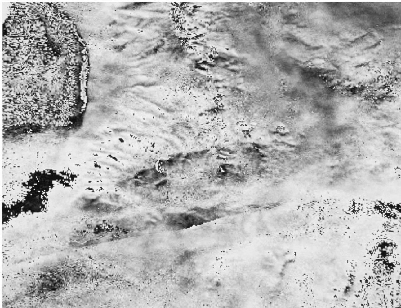
Figure 10. An interferogram showing surface rupture on the Garlock fault in California, as well as some artifactual residuals. The surface rupture appears in all the coseismic interferograms of Landers. It represents 7 \pm 4 mm of range change, projected as 19 \pm 10 mm on the ground, assuming pure horizontal displacement. Data from Massonnet et al. [1994a] as described in the caption for Plate 20a. One complete cycle of shading (from solid black to solid white) corresponds to 28 mm of range change.
