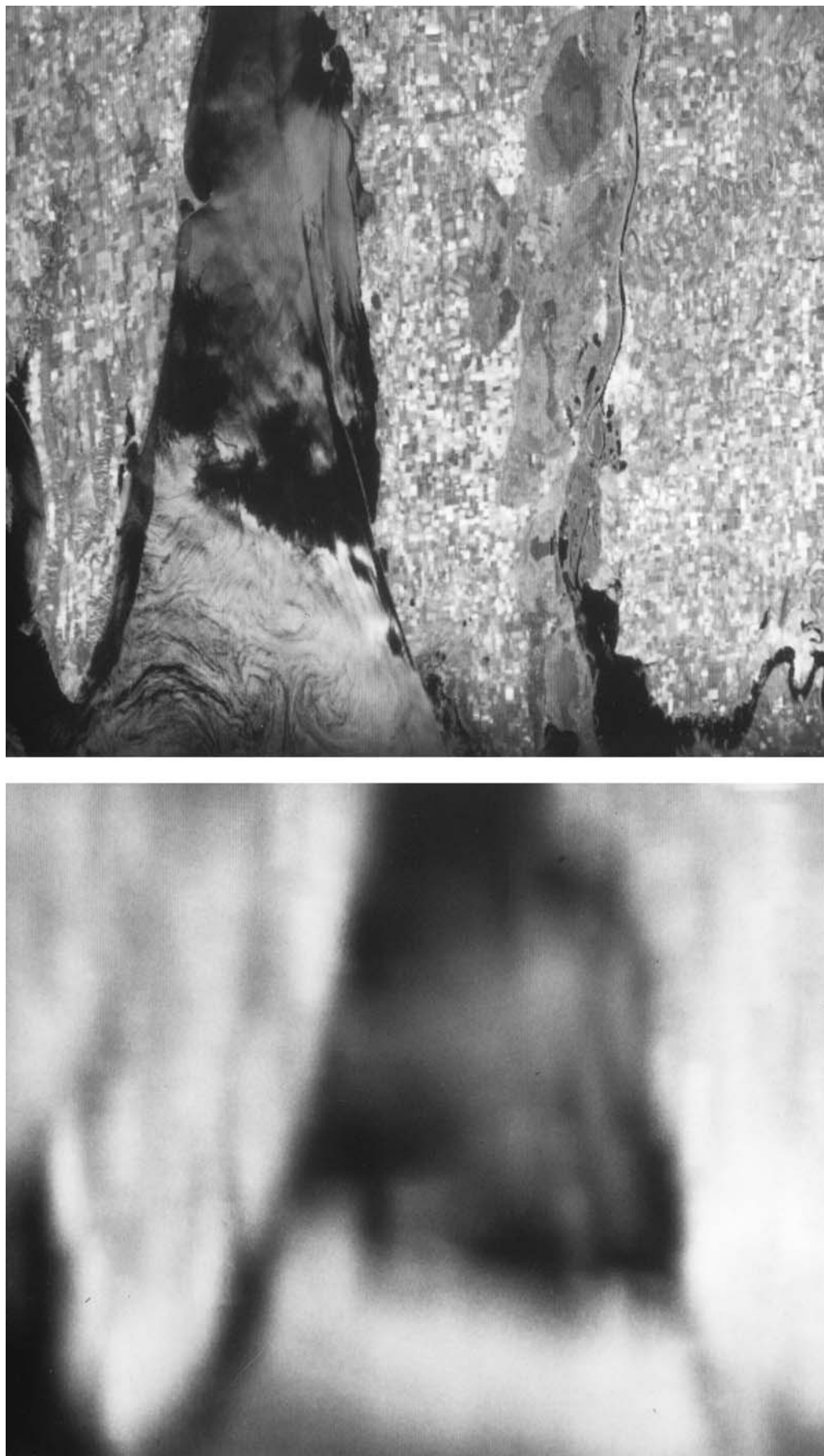
Figure 2. Improvement in resolution introduced by the synthetic aperture technique. A radar satellite “illuminates” an area with dimensions equal to the natural resolution (without synthetic aperture) of the antenna in azimuth (i.e., along the track) and the width of the electromagnetic pulse in range (i.e., across the track). On the ground these values give a resolution of about 5 km in azimuth and 14 km in range for ERS. These values are also typical of other spaceborne radar systems. The left panel shows the amplitude image of a full 100 \times 100 km frame acquired by ERS-1 over Crimea (southern Ukraine) as it was transmitted to the ground receiving station at Toulouse, France, on September 25, 1991, at \sim 2300 LT. In this image, the eye can barely distinguish the land from the sea. The synthetic aperture process leads to the full-resolution image on the right. The sea appears bright where its surface is ruffled by wind and is dark in the lee of the coast.
