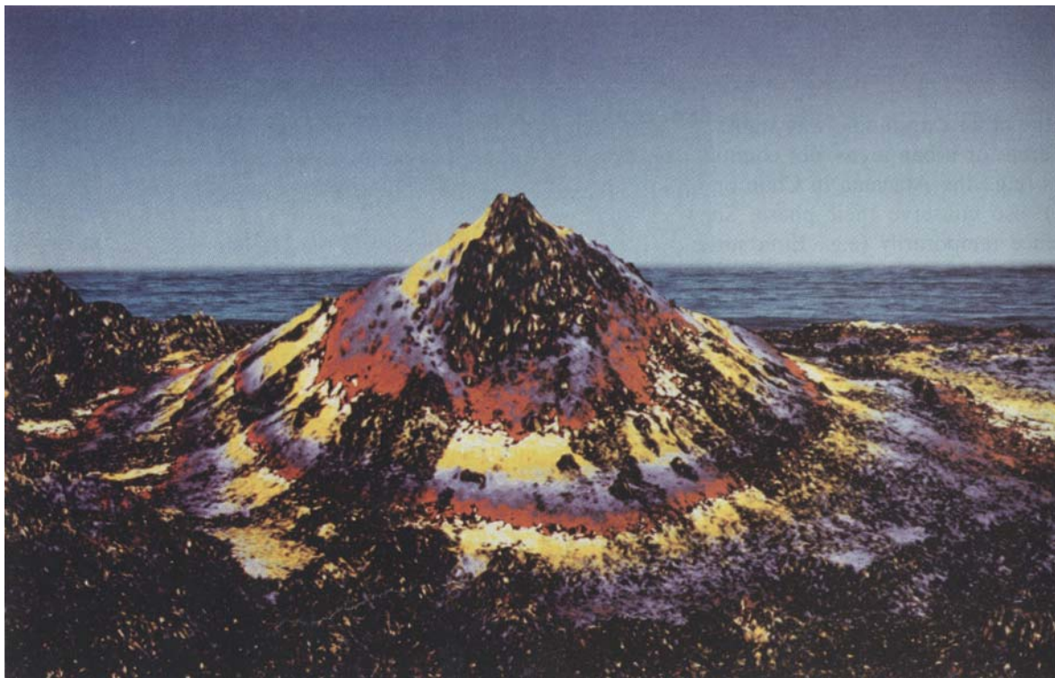
Plate 4. Mount Etna shown in perspective with its 1-year post-eruptive deformation [Massonnet et al. , 1995a]. Up to four fringes (11 cm) of deformation can be seen, with only two on the volcano proper. This example illustrates how displacement fringes can be misinterpreted as topographic fringes or vice versa. In this case the number of fringes is not proportional to topographic elevation. Furthermore, we used a DEM calculated from optical, not radar, images and tested it against an interferogram without displacements.
