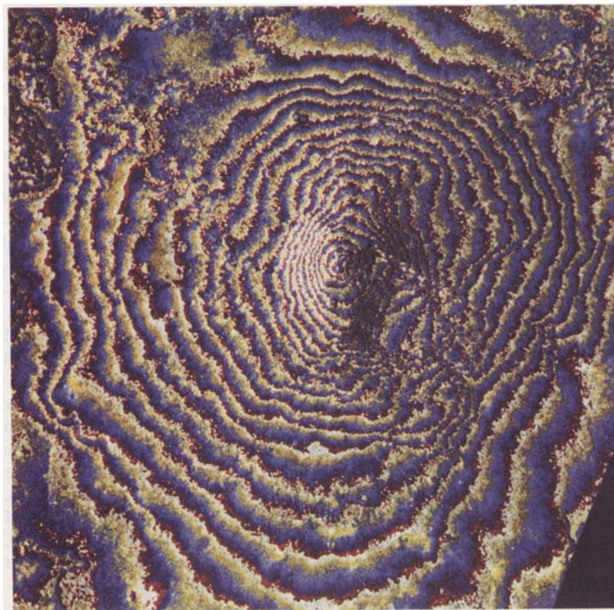
Plate 2. Topographic fringes on Mount Etna. The usual CNES processing has been altered to leave topographic fringes uncorrected while transforming the geometry to map coordinates. Here one fringe represents about 250 m of topographic elevation. The shading represents the topographic relief from the DEM, as if the illumination came from the west. The area is roughly 40 by 40 km.
