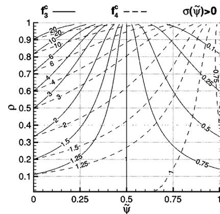
FIG. 8. Unstable  $(\tilde{\psi}, \rho)$  region (the whole plane) according to the criterion  $\sigma(\tilde{\psi}) > 0$ . The solid and dashed lines represent the bounds of the centrifugally unstable  $f$  intervals:  $f_3^c < f < f_4^c$ .
