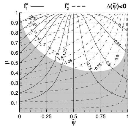
FIG. 7. Unstable  $(\tilde{\psi}, \rho)$  region (in white) according to the criterion  $\Delta(\tilde{\psi}) < 0$ . The solid and dashed lines represent the bounds of the unstable  $f$  intervals:  $f_1^c < f < f_2^c$ .
