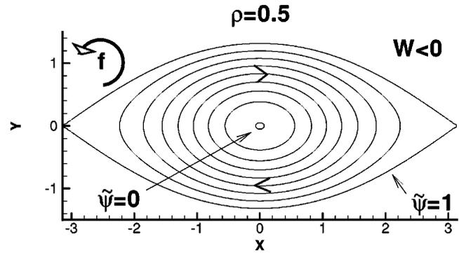
FIG. 3. Streamlines of the Stuart vortices for  $\rho=0.5$ . The flow is periodic in the  $x$  direction with period  $2\pi$ .
