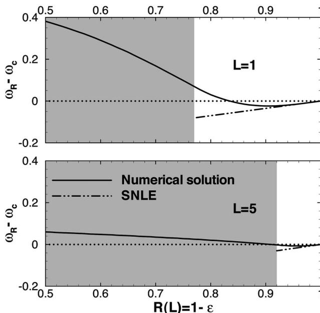
FIG. 2. Value of  $\omega_R - \omega_c$  ( $\omega_R$  being the swirl at which a wall recirculation is obtained) as a function of the exit duct radius  $R(L)$ , for  $L=1$  and  $L=5$ . Comparison between the SNLE [valid in the vicinity of  $R(L)=1$ ] and the numerical solution. In the shaded region, the recirculation is obtained for  $z < L$ , inside the duct.
