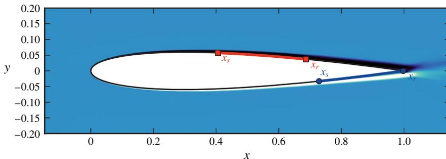
FIGURE 1. (Colour online) Mean flow considered in the present study, visualised by the streamwise velocity component. The boundary layer on the suction surface detaches between  $x_s \approx 0.405$  and  $x_r \approx 0.686$ , while the pressure-surface boundary layer detaches between  $x_s \approx 0.728$  and  $x_r \approx 0.977$ . The reader is referred to Fosas de Pando *et al.* (2014) for further details on the mean-flow characteristics.
