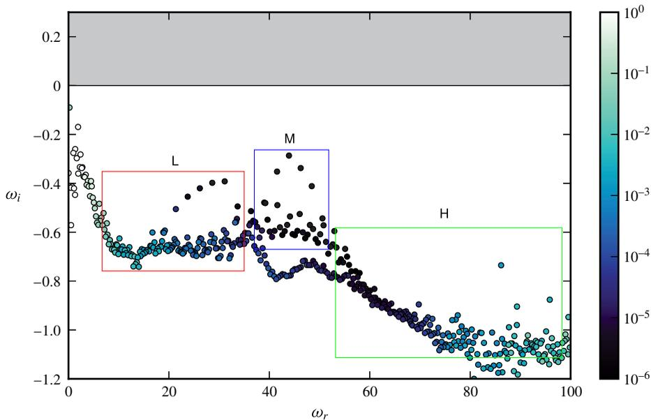
FIGURE 2. (Colour online) Global spectrum of the tonal noise problem in the complex frequency plane. The eigenvalues are coloured according to the size of the relative residual with respect to the operator  $\mathbf{A}$ . The spectrum is divided into least stable modes (labelled M), low-frequency modes (labelled L) and high-frequency modes (labelled H).
