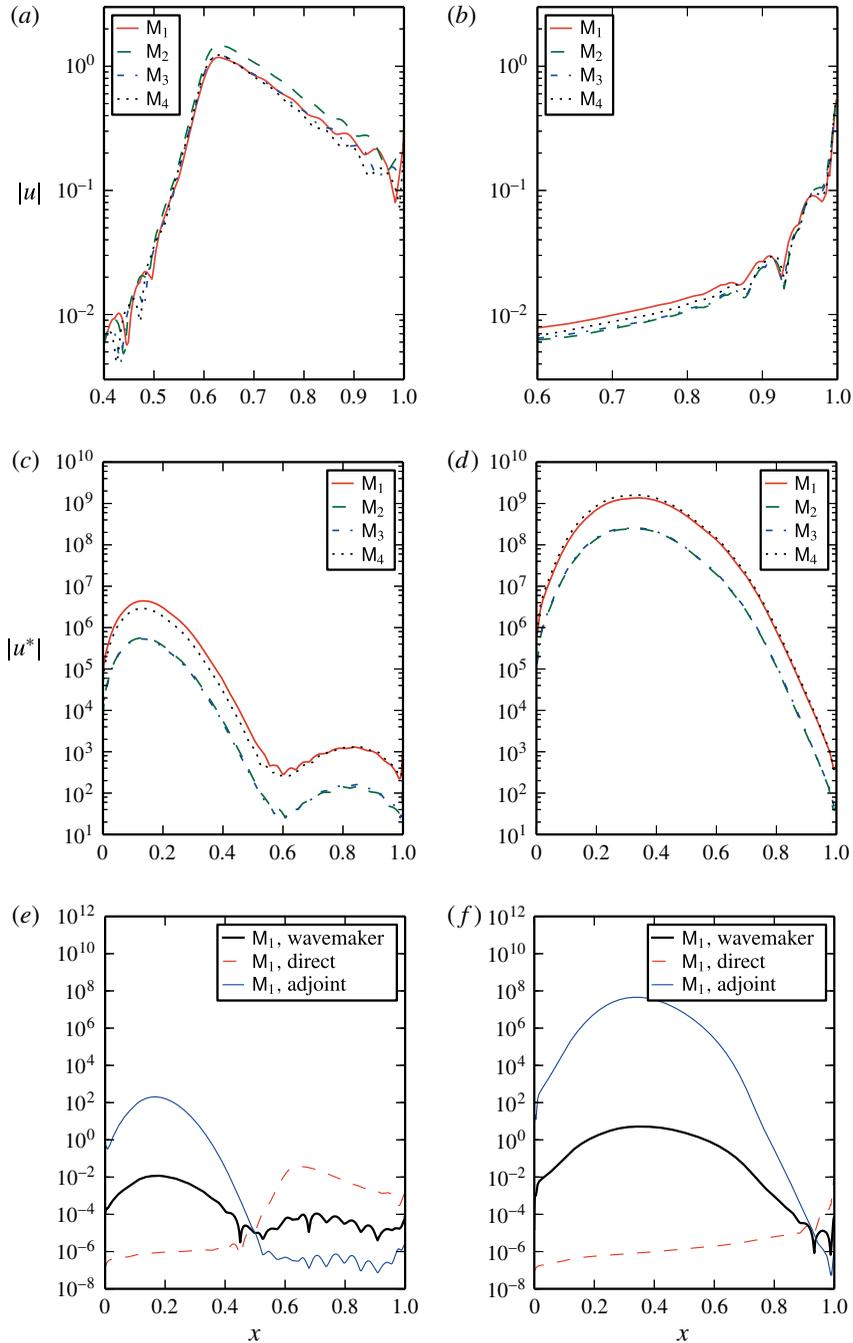
FIGURE 5. (Colour online) Evolution of the streamwise velocity peak along the aerofoil chord (a) on the suction surface and (b) on the pressure surface of the aerofoil for the leading modes labelled  $M_1$ – $M_4$  in figure 3. (c,d) Same for the adjoint streamwise velocity peak. (e,f) Same for the direct mode, adjoint mode and wavemaker corresponding to  $M_1$ .
