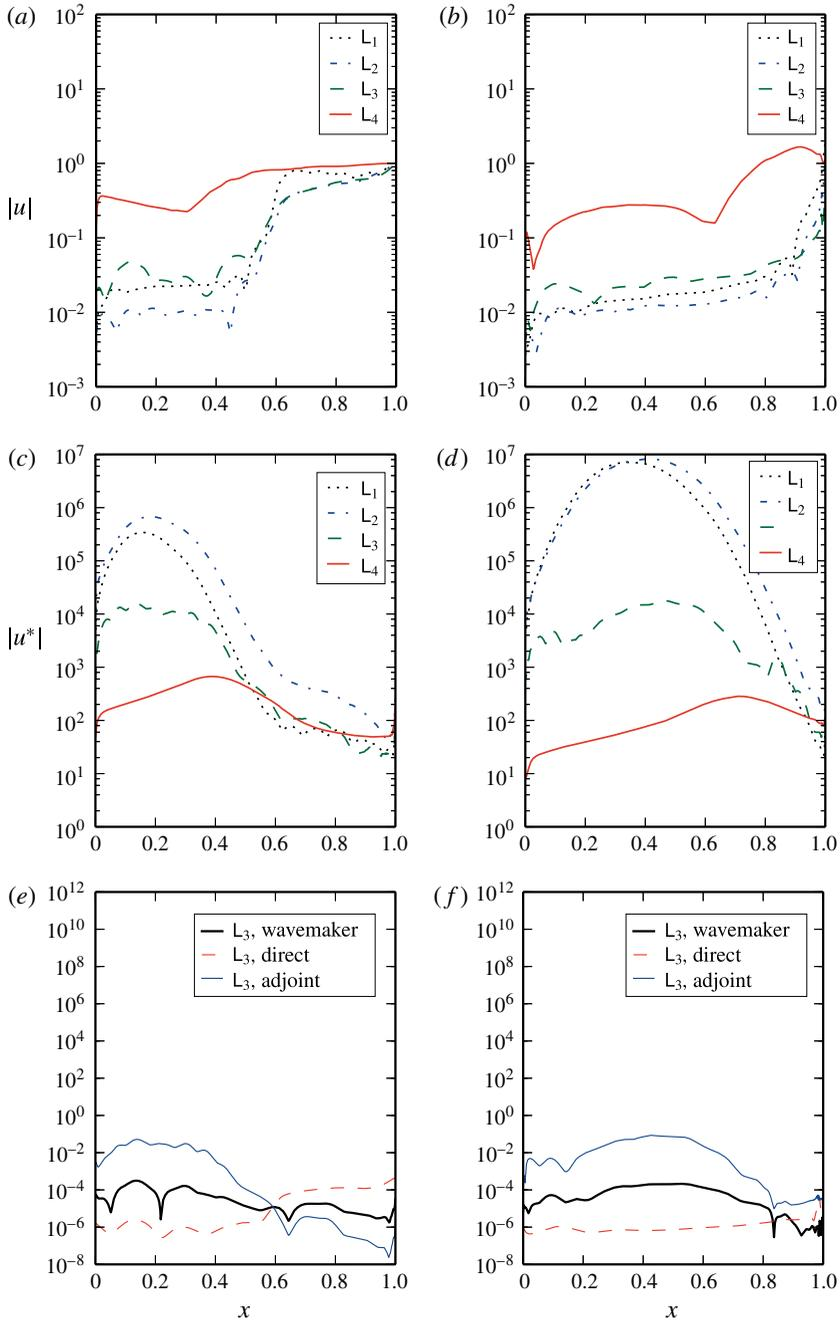
FIGURE 11. (Colour online) Evolution of the streamwise velocity peak along the aerofoil chord (a) on the suction surface and (b) on the pressure surface of the aerofoil for the low-frequency modes labelled  $L_1$ – $L_4$  in figure 9. (c,d) Same for the adjoint streamwise velocity peak. (e,f) Same for the direct mode, adjoint mode and wavemaker corresponding to  $L_3$ .
