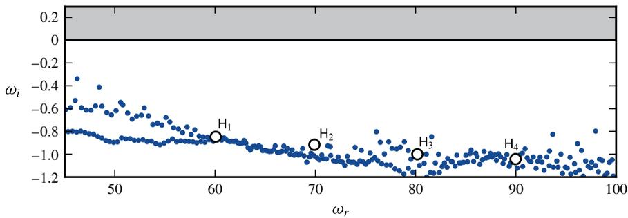
FIGURE 6. (Colour online) Global spectrum displaying high frequencies  $\omega > 45$ ; the modes labelled  $H_1$ – $H_4$  will be analysed further. Their associated eigenfrequencies are:  $\omega_{H_1} = 60.06 - 0.85i$ ,  $\omega_{H_2} = 69.90 - 0.92i$ ,  $\omega_{H_3} = 80.17 - 1.00i$ , and  $\omega_{H_4} = 89.97 - 1.05i$ . The residual associated with the iterative eigenvalue solver is smaller than  $5 \times 10^{-3}$ .
