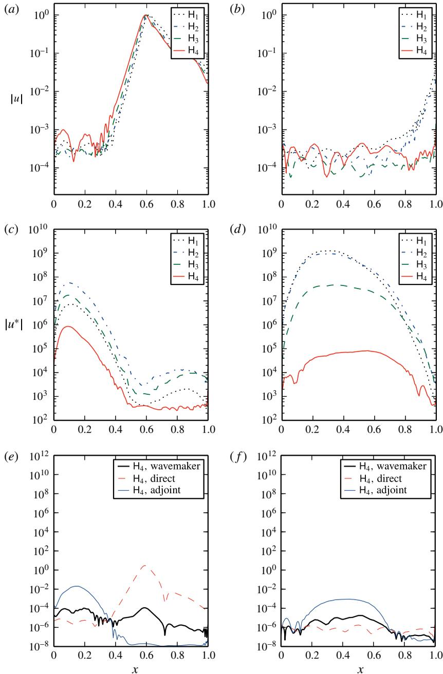
FIGURE 8. (Colour online) Evolution of the streamwise velocity peak along the aerofoil chord (a) on the suction surface and (b) on the pressure surface of the aerofoil for the high-frequency modes labelled  $H_1$ – $H_4$  in figure 6. (c,d) Same for the adjoint streamwise velocity peak. (e,f) Same for the direct mode, adjoint mode and wavemaker corresponding to  $H_4$ .
