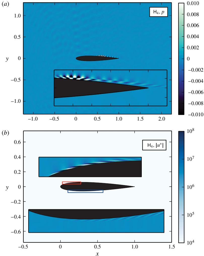
FIGURE 7. (Colour online) Direct and adjoint global mode corresponding to  $H_4$  indicated in figure 6, visualised by the real part of the pressure field (a) and absolute value of the adjoint streamwise velocity (b). The insets, showing the real part of the streamwise velocity, give more details of the respective flow fields.
