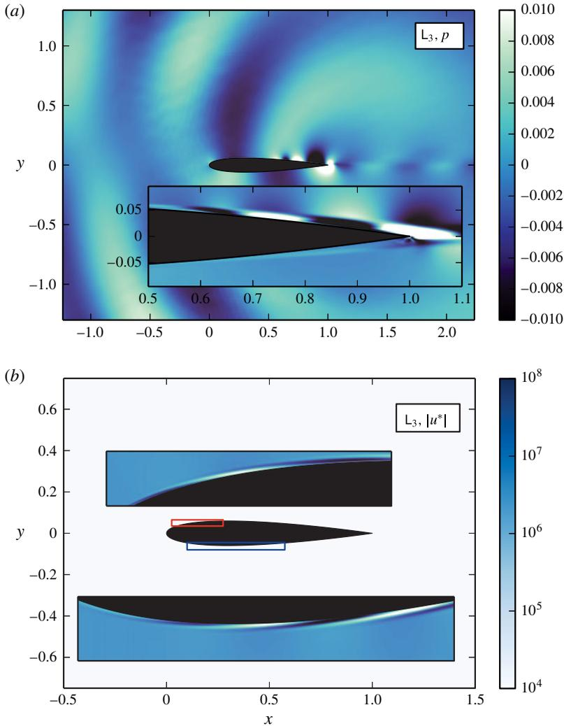
FIGURE 10. (Colour online) Direct and adjoint global modes corresponding to  $L_3$  indicated in figure 9, showing streamwise velocity (a) and adjoint streamwise velocity (b). The insets give more details of the respective flow fields.
