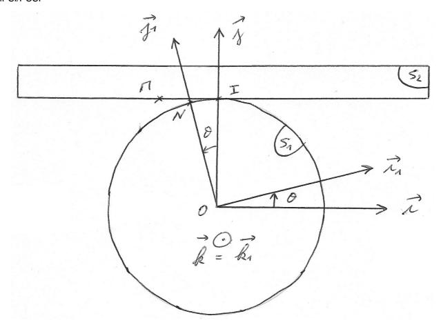
Composition de mouvement :  $\vec{V}(I \in S2/S1) = \vec{V}(I \in S2/S0) + \vec{V}(I \in S0/S1)$
