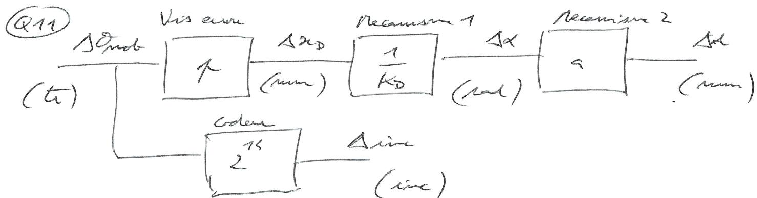
$$\text{Pour 1 mecanism} \Rightarrow \Delta l = \frac{a}{K_D} \frac{\pi}{2^{15}} = \frac{0,183}{0,022} \times \frac{\pi}{2^{15}} =$$
