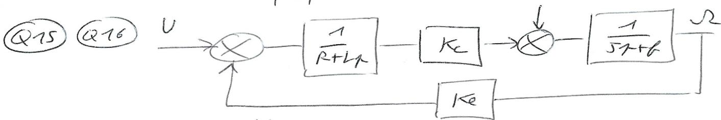
$$Q17 F_{m1} = \frac{\frac{K_c}{R_f + K_c K_e}}{\frac{LJ}{R_f + K_c K_e} s^2 + \frac{2f + RS}{R_f + K_c K_e} s + 1}$$
