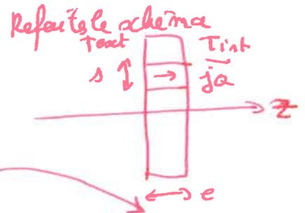
De plus,  $P_{th} = \frac{T_{ext} - T_{int}}{R_{th}}$  donc  $\frac{\Delta T}{R_{th}} = -\lambda \frac{\partial T}{\partial x} S = P_{th}$   $\left. \begin{array}{l} \\ \\ \end{array} \right\} \frac{dT}{dx} = \frac{T_{int} - T_{ext}}{e}$
