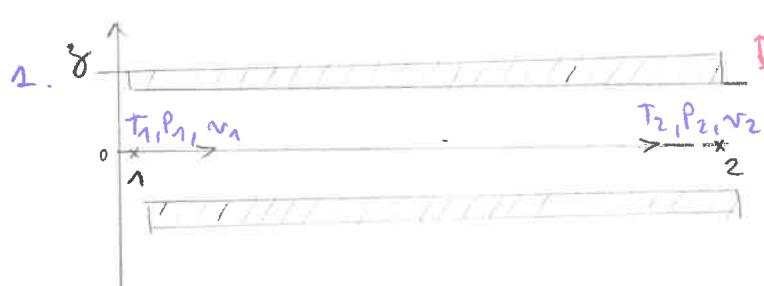
$$Dm \left[ (h_2 - h_1) + (e_{c2} - e_{c1}) + (e_{p2} - e_{p1}) \right] = P_{mica} + P_{th}$$
