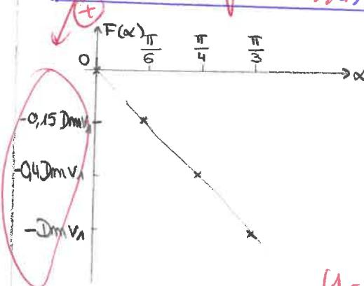
$$F(\frac{\pi}{6}) = Dm v_2 (1 - \frac{2}{\sqrt{3}}) = -0.15 Dm v_2$$
