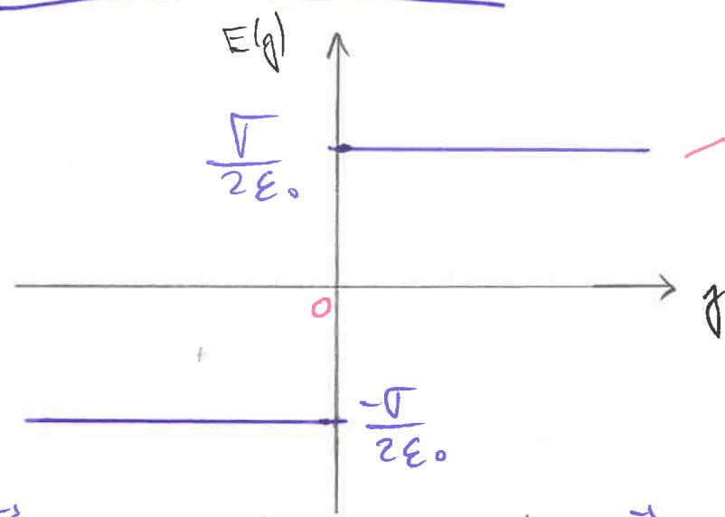
$$\begin{aligned} dV &= -\vec{E} \cdot d\vec{l} = (-E(y)\vec{u}_y) \cdot (dx\vec{u}_x + dy\vec{u}_y + dz\vec{u}_z) \\ &= -dy E(y) \end{aligned}$$
