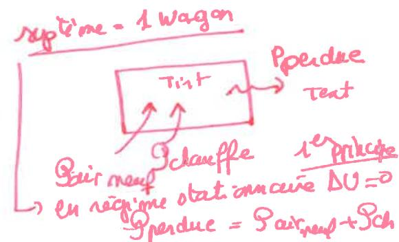
$$\rightarrow P_{ch} = \frac{T_2 - T_1}{R_{th}} - P_{air \text{ neuf}} \quad \text{avec } P_{air \text{ neuf}} = Dm \cdot C_p (T_{int} - T_{ext})$$
