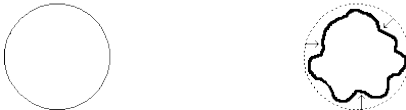
to maintain a constant surface area when deformed, a spherical shape must necessarily contract the overall volume it occupies
